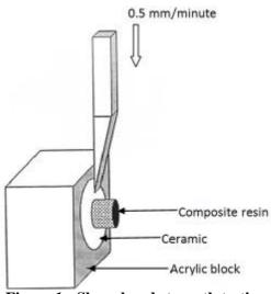
Figure 1: Shear bond strength testing
