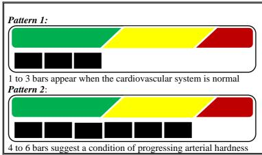
Figure 1: H-Value measurement result on the LCD Display of ASI measuring device
