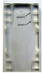
Figure 1: The clear block with simulated curved root canals
