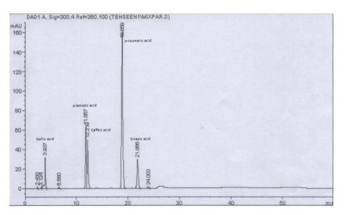
Fig. 1: A typical RP-HPLC chromatogram of mixture of phenolics acid standards. Peak identification: 1: gallic acid (RT 3.96), 2: *p*-hydroxyl benzoic acid (RT 11.97), 3: caffeic acid (RT 12.44), 4: *p*-coumeric acid (RT 19.04), 4: sinapic acid (RT 22.13)
