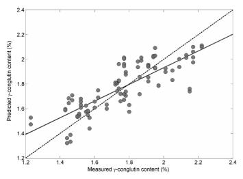
Fig. 1: Scatter plot of measured vs. predicted seed γ-conglutin content (in % w/w) for 46 genotype-environment combinations. Prediction based on a Near-Infrared Reflectance spectroscopy calibration curve, using cross-validations (continuous line = regression line; broken line = 1:1 line)
