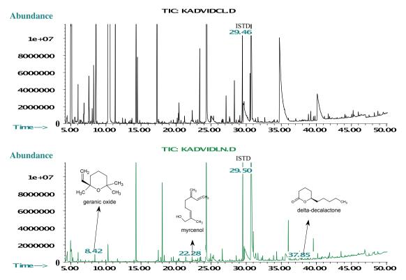
Fig. 1: The TICs of the Szekszárdi Kadarka wine samples, simple distillation followed by LLE extraction (upper), LN-SDE extract (lower)
