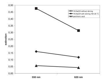
**Fig. 2:** Extinction of the amylose iodine and the amylopectin iodine complex at 620 and 550 nm using different solvents for whole grains.
