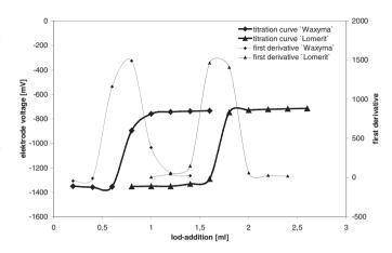
Fig. 1: Amperometric titration curves and first derivative of the waxy barley 'Waxyma' and the standard barley 'Lomerit'.
