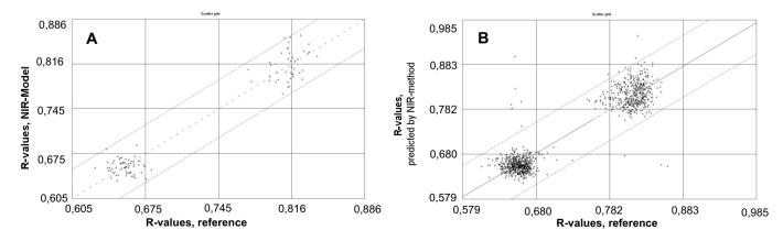
Fig. 3: A: Correlation between NIT-spectra data and chemical analysis data (R-values) determined by the two-wavelength colorimetric method in single kernels.
