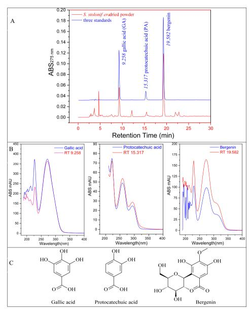
Fig. 2: HPLC-DAD patterns of three standards (GA, PA and bergenin) and the main components in S. stolonifera (A). UV spectra (B) and their molecular structures (C) of three standards and three peaks in S. stolonifera. RT: retention time of three peaks in HPLC-DAD.
