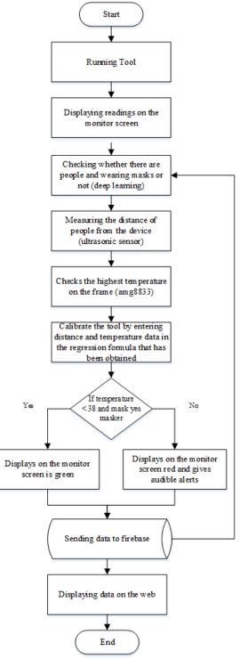
Figure 4. Tool workflow
