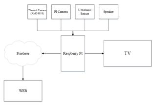
Figure 5. Tool architecture
