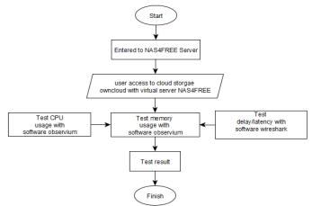
Figure 4. NAS4FREE virtual server test flowchart
