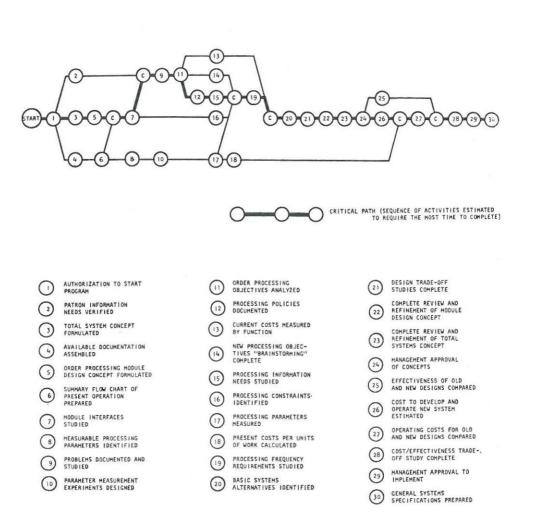
Fig. 6. System Development Program (PERT) Planning Diagram.
