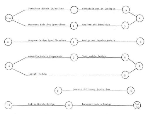
Fig. 8. Generalized Module Development Planning Network.
