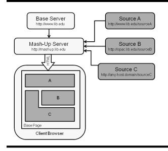
Figure 1. Server-side mash-up construction
