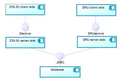
**Figure 1.** Software Architecture of a System with Separate Implementations of Server-Side Protocols
