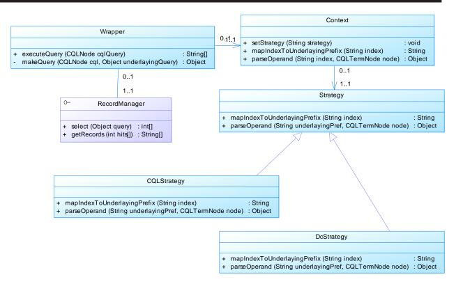
Figure 7. UML Class Diagram of Wrapper Component
