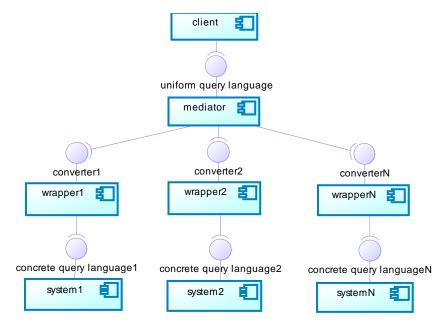
Figure 3. Architecture with the Mediator/Wrapper Approach
