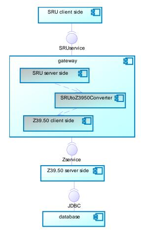
Figure 2. Software Architecture of a System with a Gateway
