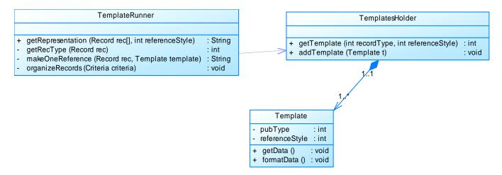
Figure 3. Architecture of the component for generating template.
