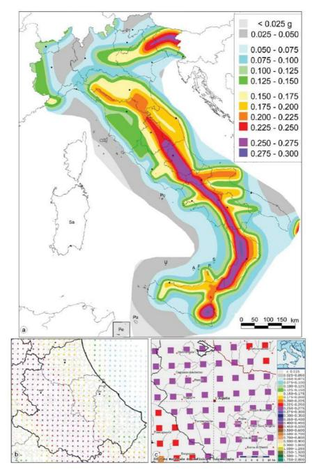
Figure 4 – Seismic Hazard Map of (a) Italy, (b) Abruzzo region and (c) L'Aquila area (c) (from INGV, 2004), in terms of ground peak acceleration with 10% excess probability in 50 years, referred to rigid bedrock (Vs30>800 m/s).
