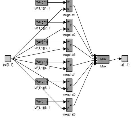
Fig. 3. A neural network structure represented by blocks Simulink
