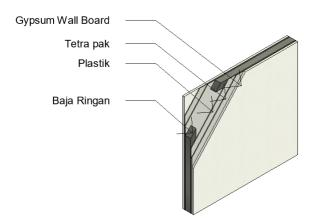
Figure 3. Application of tetra pack on the walls of buildings
