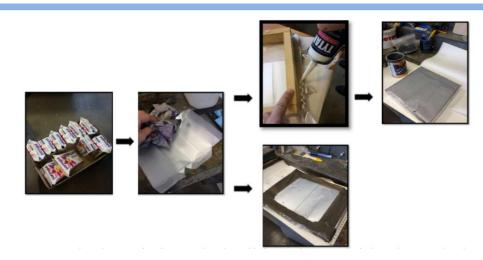
Figure 1. The process of making tetra pack layers
