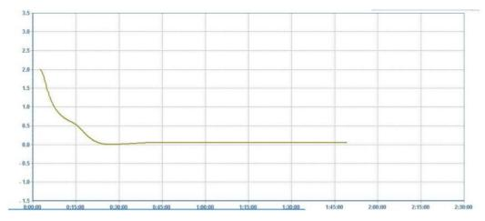
**Figure 3**. Graphic obtained from the Guarded Hot Plate Test for Stacked TetraPak Packages (time x thermal conductivity)
