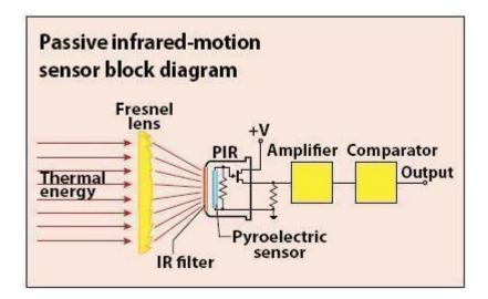
Figure 1. PIR sensor movement diagram
