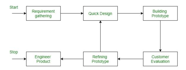
Figure - Prototype Model
