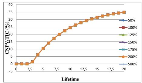
Figure 7. Effect of utility variation on CNPV/TIC with 20 years of service life.
