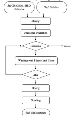
Figure 1. Schematic process on the production of ZnS nanoparticles
