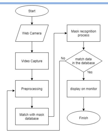
Figure 2. Mask Detection Flow Chart
