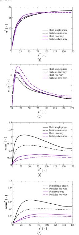
Figure 2. Non-dimensional fluid and particle mean and fluctuating velocities for oneway and two-way coupling conditions: a) stream-wise mean velocity, b) stream-wise rms velocity, (c) span-wise rms velocity, (d) wall-normal rms velocity Source: Authors
