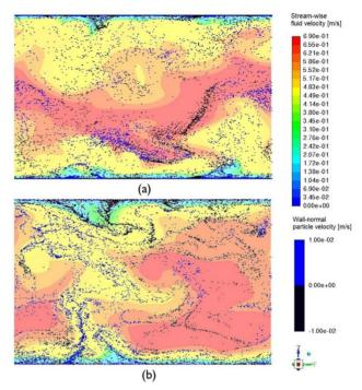
Figure 7. Illustration of the stream-wise velocity field in the middle stream-wise plane under one-way coupling (a) and two-way coupling (b) configurations. Positions of particles around that plane are shown as colored dots. Black dots represent particles with negative wall-normal velocities, whereas blue dots denote particles with positive wall normal velocities. Flow is orthogonal to the plane.
