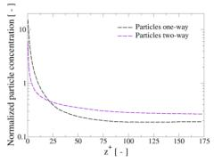
Figure 3. Normalized particle concentration profiles for one-way and two-way coupled simulations
