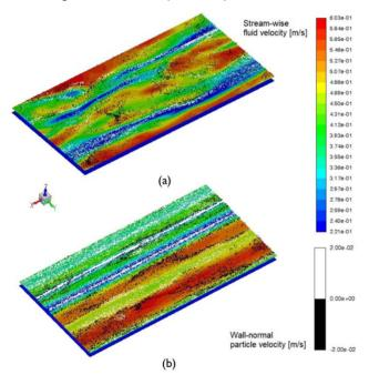
**Figure 6.** Illustration of the velocity field in the plane  $z^+ = 18$  within the buffer layer under one-way coupling (a) and two-way coupling (b) configurations. Positions of particles around that plane are shown as colored dots. Black dots represent particles moving towards the wall, whereas white dots denote particles escaping from the wall. Flow is in the positive x-direction. **Source:** Authors
