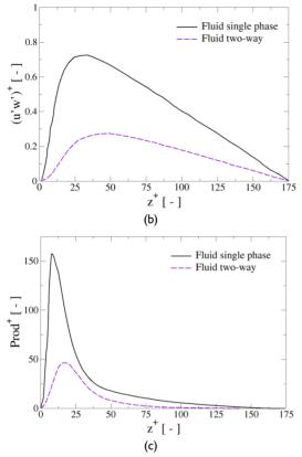
Figure 4. Non-dimensional fluid turbulent kinetic energy (a), turbulent shear stresses (b), and turbulent kinetic energy production term (c) for single phase and two-way coupling conditions
