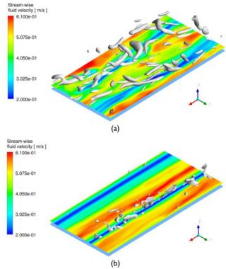
Figure 5. Illustration of the velocity field in the plane  $z^+=18$  within the buffer layer. The turbulent structures identified by the Q criterion are included. a) Single phase flow,  $Q=50\ s^{-2}$ ; (b) two-phase flow,  $Q=10\ s^{-2}$ . Flow is in the positive x-direction.
