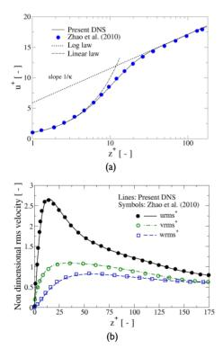
**Figure 1.** Non-dimensional velocity (a) and rms velocity profiles (b) for the single-phase flow. Comparison with Zhao *et al.* (2010). The theoretical linear and logarithmic laws are also shown in (a).
