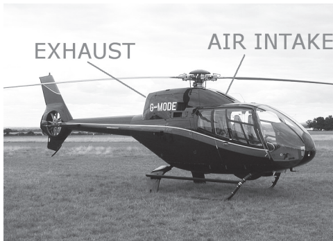
Figure 5. Air intake and exhaust in the turbine powered helicopter.
