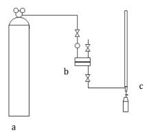
Figure 1: Gas permeation test cell; (a) gas silinder, (b) membrane cell, (c) buble soap
