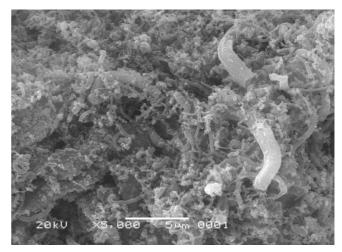
Figure 2: Carbon nanotubes surface with no modification
