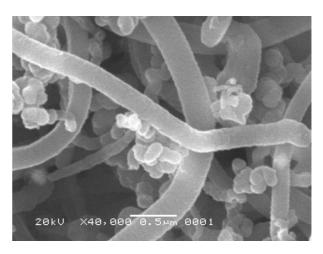
Figure 3: Carbon nanotubes surface with modification
