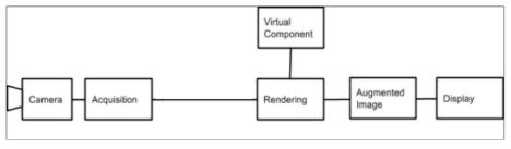
Fig. 2. Augmented Reality Flow
