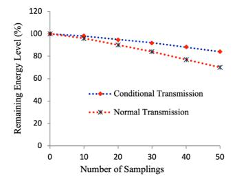
Fig. 3. Energy level comparison with respect to number of samplings
