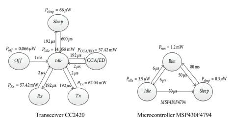
Fig. 2. Performance analysis of state transition in WSN node
