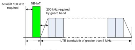
Fig. 6. NB-IoT deployment on LTE idle spectrum resources
