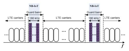
Fig. 7. LTE guard band deployment
