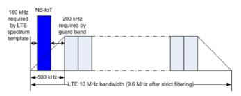
Fig. 8. LTE guard band deployment
