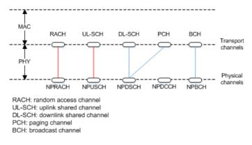
Fig. 2. Mapping relationships between physical channels and transport channels
