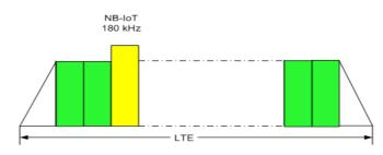
Fig. 9. LTE In-band deployment
