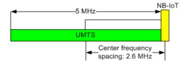
Fig. 5. NB-IoT deployment on UMTS idle spectrum resources
