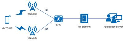
Figure 4 illustrates the end-to-end network architecture of eMTC.
