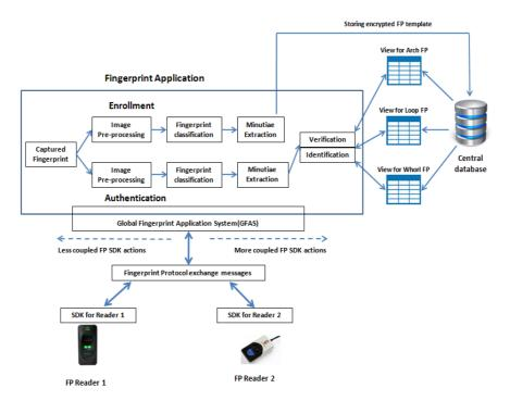
Fig. 3. Architecture of the proposed system
