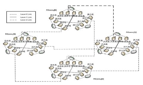
Fig. 5. A FiConn Interconnection Structure with n = 4 [28]
