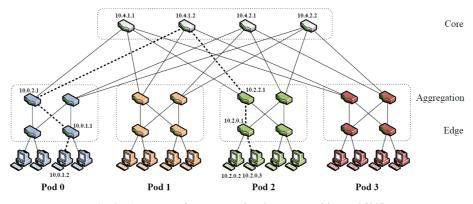
Fig. 2. A Fat-Tree interconnection Structure, with n = 4 [22]
