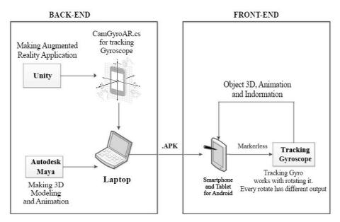
Fig. 1. Schematic of System Development
