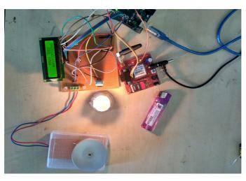
Fig. 11.Cool down process Initialized when temperature is raised
