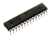
Fig. 4. ATMEGA 328P AVR Microcontroller [3]
