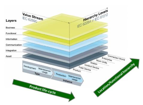
Fig. 5. Reference Architecture Model for Industry 4.0 [11]
