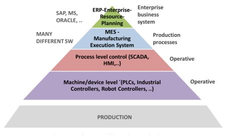
Fig. 3. Automation pyramid in modern production systems
