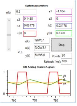
Fig. 11. PLC system representing the ARX(2,2,1) and the I/O.
