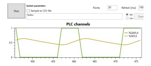
Fig. 10. PLC chart showing the output and input of the system.
