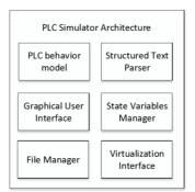
Fig. 5. Local PLC application architecture.
