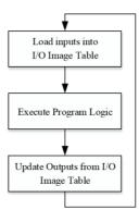
Fig. 4. Application scan cycle [21].
