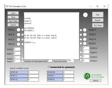
Fig. 3. Local virtual PLC framework graphical user interface.
