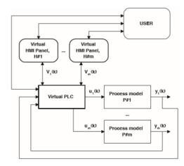
Fig. 7. Example of supervision/control architecture of the PLC simulator.
