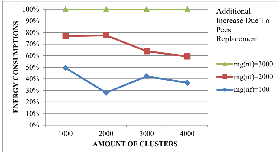
Fig. 7. When mg = 2000 , the power usage of PECS is determined by the number of clusters
