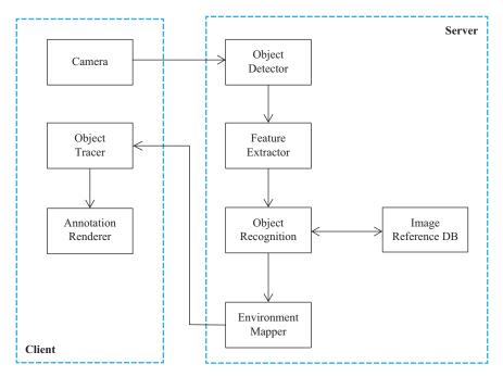
Fig. 1. Simple pipeline structure of the MAR
