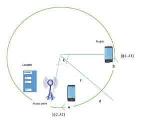
Fig. 1. Distance calculation on the surface of sphere
