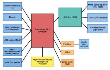
Fig. 1. System architecture
