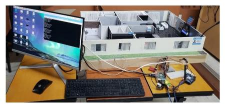
Fig. 4. Prototype gas leak detection and surveillance system
