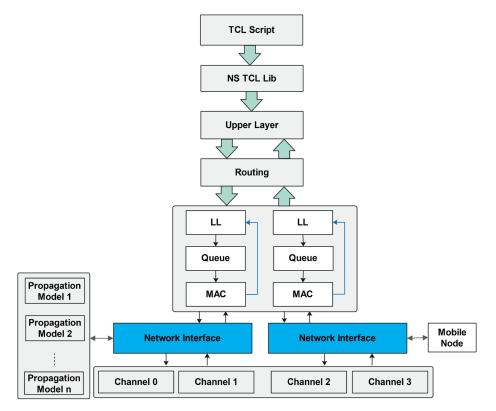
Fig. 3. Multi-channel multi-interface wireless node architecture in NS2
