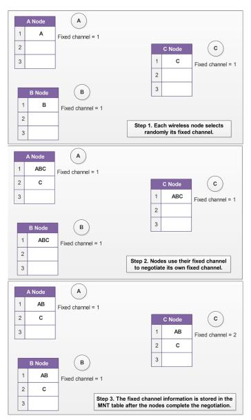
Fig. 4. The three-step negotiation process determines the fixed channel of the wireless nodes in the WMN
