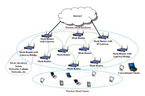
Fig. 2. An illustration of the Hybrid WMN architecture
