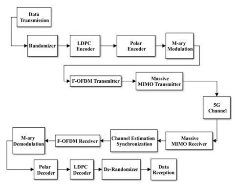
Fig. 1. Basic physical layer architecture of 5G system
