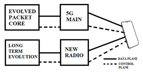
Fig. 2. Standalone architecture of 5G communication
