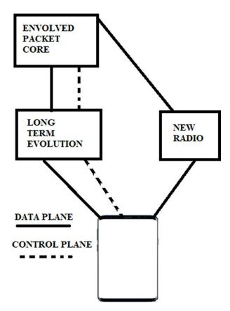
Fig. 3. Non-Standalone architecture of 5G communication
