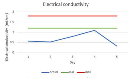
Fig. 11. Electrical conductivity in case without control
