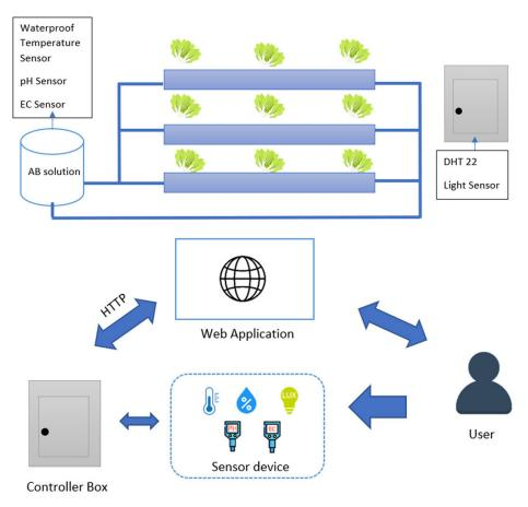
Fig. 2. Common sensors in hydroponics systems
