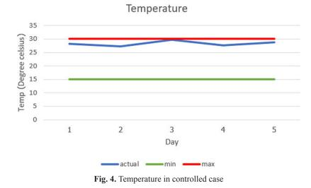
The optimum temperature for plants for a controlled hydroponics system shows that the average intraday value is within the optimum range. There will be some days when the graph goes up to the highest value because of the heat from the artificial lights that we have turned on as shown in Figure 5. However, the duration of light received by the plant may be insufficient for photosynthesis. Water temperature, in addition to room temperature, is required for plant growth.
