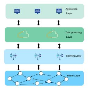
Fig. 3. Four-layer architecture of a sensor network
