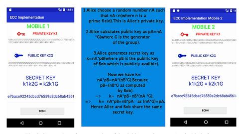
Fig. 8. Screen shot of secure and confidential key exchange on Android platform
