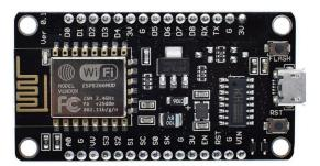
Fig. 1. NodeMCU v3 board structure
