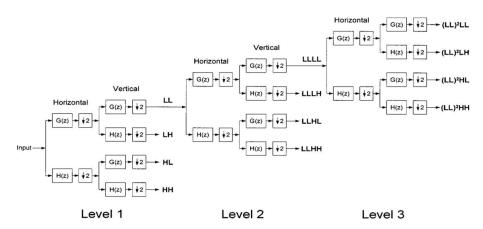
Fig. 2. Three-level Discrete Wavelet Transform
