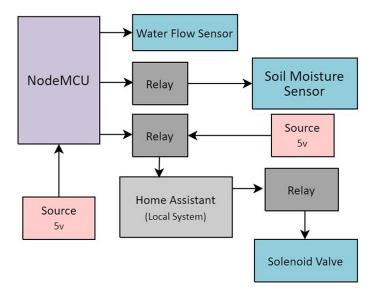
Fig. 9. Design of the NodeMCU and Home Assistant option
