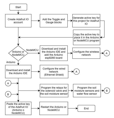
Fig. 7. Adafruit IO, Arduino, and NodeMCU process diagram
