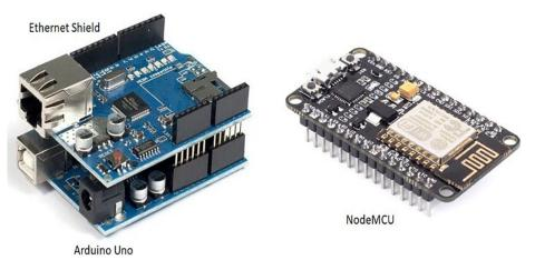
Fig. 4. Plate alternatives used for irrigation automation
