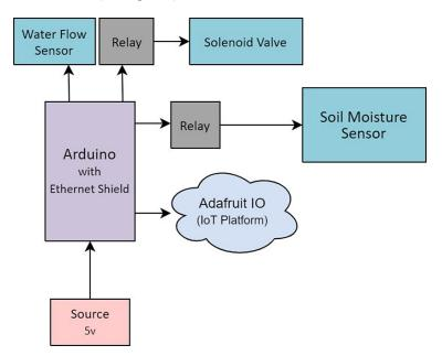
Fig. 5. Design of the option with Arduino and Adafruit IO
