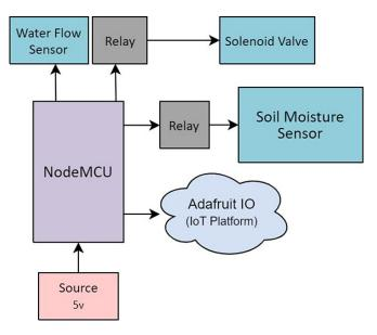
Fig. 6. Design of the option with NodeMCU and Adafruit IO
