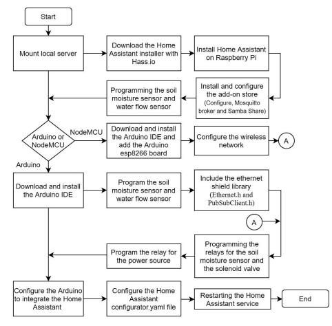
Fig. 10. Home Assistant, Arduino, and NodeMCU process diagram
