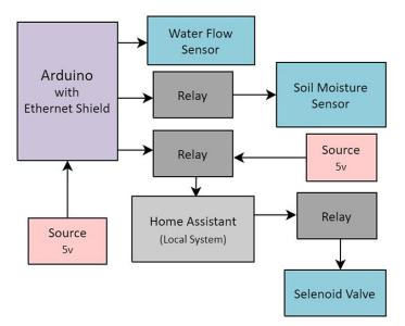
Fig. 8. Design of the Arduino and Home Assistant option
