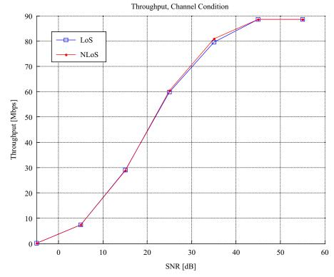
Fig. 3. Comparison between LoS and NLoS channel for the proposed IBCQI
