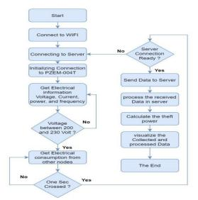
Fig. 5. The flowchart of an electrical energy management system based on IoT
