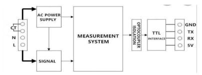
Fig. 4. The block diagram of pzen-004t
