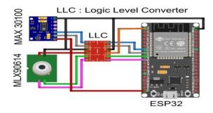
Fig. 6. The circuit connection between the sensors and microcontroller
