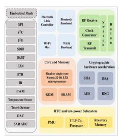
Fig. 3. The block diagram of ESP32.
