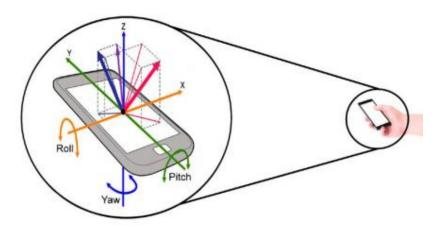
Fig. 4. IMU sensor measurement
