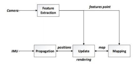
Fig. 2. SLAM pipeline scheme
