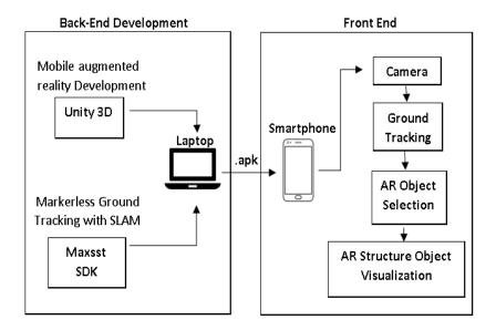
Fig. 1. Mobile augmented reality scheme
