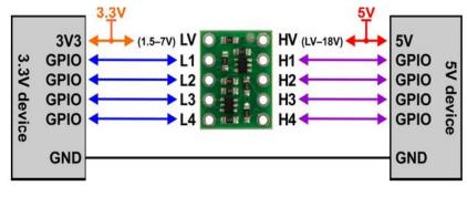
Fig. 7. Logic Level Converter.
