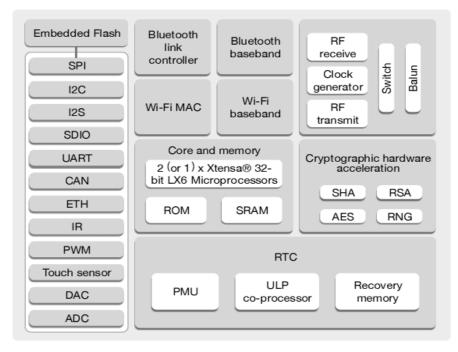
Fig. 6. The block diagram of the ESP3
