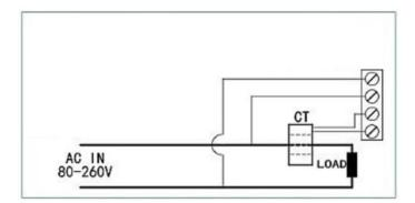
Fig. 4. The wiring diagram of the PZEM-004t
