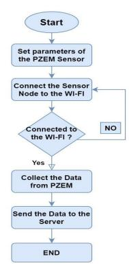
Fig. 8. IoT-based Modbus EMS flow chart
