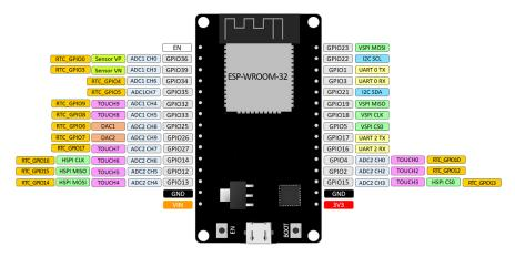
Fig. 5. The ESP32 microcontroller
