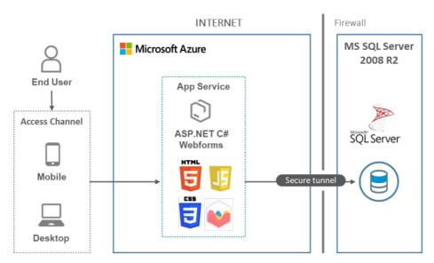
Fig. 4. Platform Architecture of A Mobile Web
