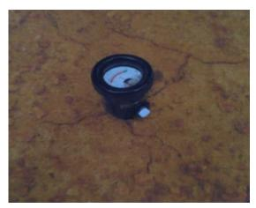
Figure 8. pH Top Soil Measurement
