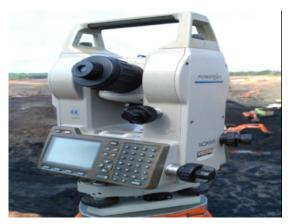
Figure 3. Total Station Set Survey Tool 3010
